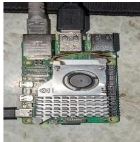
Fig 2 -Raspberry Pi 5 Model B
